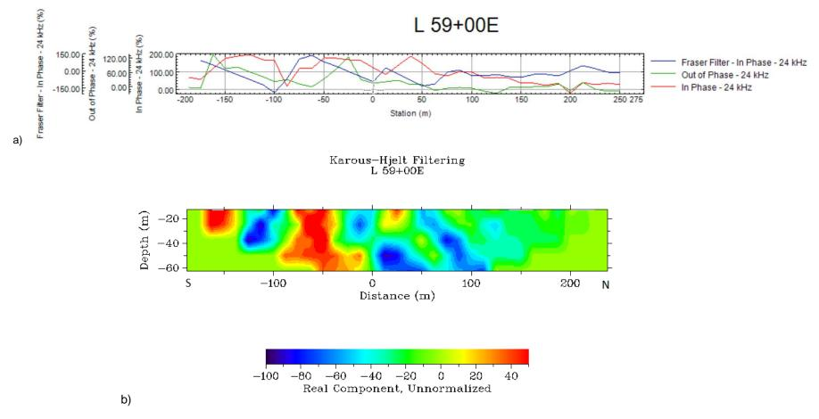
Figure 9. In-Phase, Out-of-Phase and Fraser Filter Profiles (a) Current density Pseudo-distributions obtained with Karous-Hjelt filter (b) – LinJog Lake – L 59+00E.
