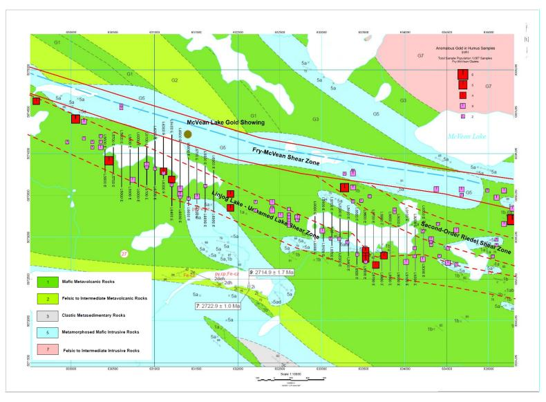
Figure 1. Geology of the Fry-McVean Project with Fry-McVean Shear Zones, Au soil anomalies and VLF-EM grids.
