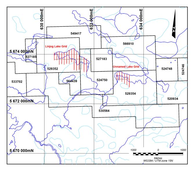
Figure 25. Index of claims and ground VLF-EM coverage (red lines) within the Fry-McVean Project.
