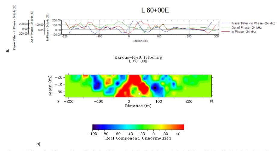
Figure 10. In-Phase, Out-of-Phase and Fraser Filter Profiles (a) Current density Pseudo-distributions obtained with Karous-Hjelt filter (b) – LinJog Lake – L 60+00E.
