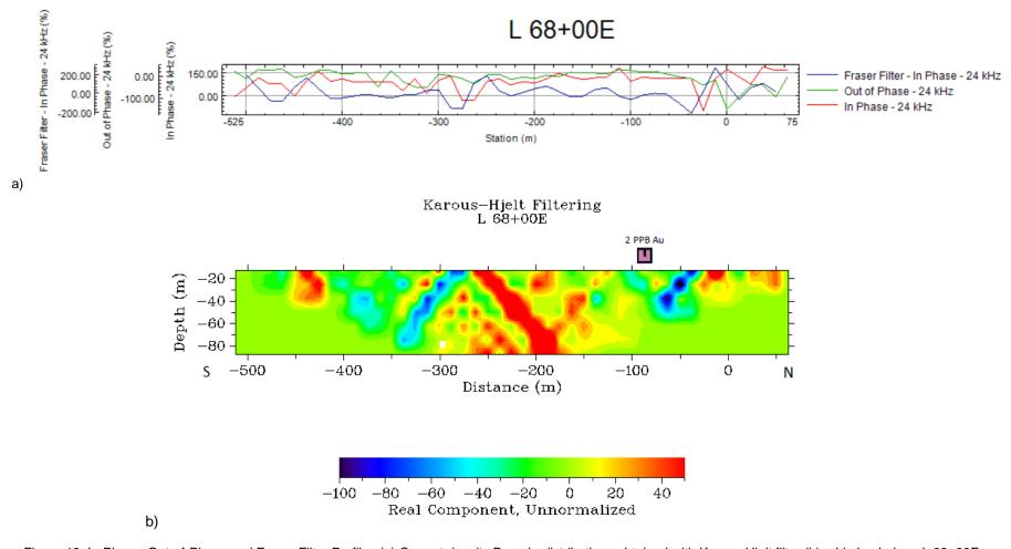
Figure 16. In-Phase, Out-of-Phase and Fraser Filter Profiles (a) Current density Pseudo-distributions obtained with Karous-Hjelt filter (b) – LinJog Lake – L 68+00E.
