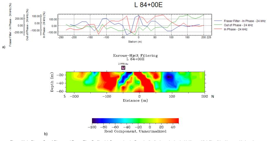
Figure 22. In-Phase, Out-of-Phase and Fraser Filter Profiles (a) Current density Pseudo-distributions obtained with Karous-Hjelt filter (b) – Unnamed Lake – L 84+00E.
