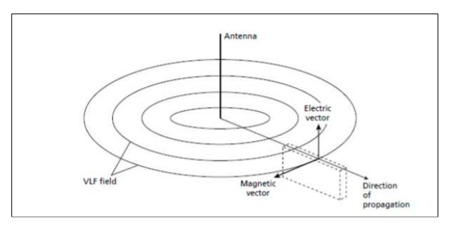
Figure 2. Principle of VLF method; dashed lines show a tabular conductor striking towards the antenna which is cut by the magnetic vector of the EM field.
