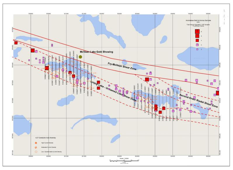
Figure 5. Fry-McVean Project with Fry-McVean Shear Zones, Au soil anomalies and VLF trends.
