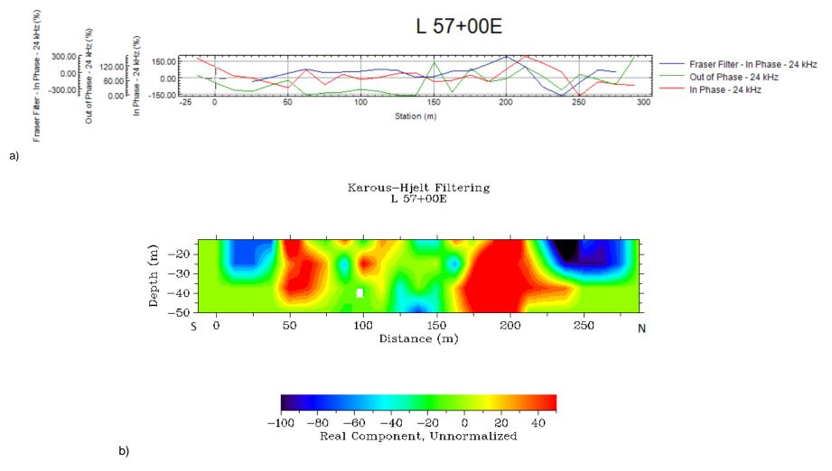
Figure 7. In-Phase, Out-of-Phase and Fraser Filter Profiles (a) Current density Pseudo-distributions obtained with Karous-Hjelt filter (b) – LinJog Lake – L 57+00E.
