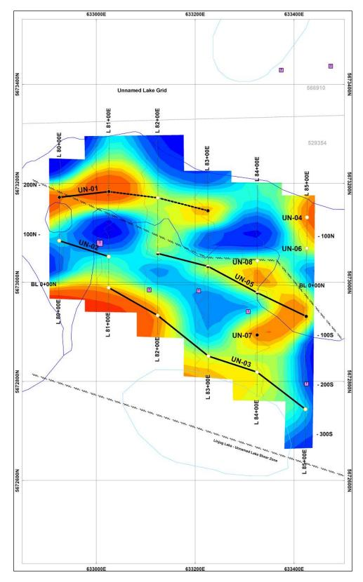
Figure 3. Fraser Filter Contours with outlined VLF Conductors – Unnamed Lake
