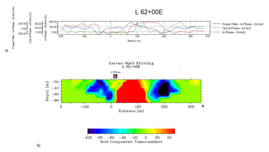
Figure 12. In-Phase, Out-of-Phase and Fraser Filter Profiles (a) Current density Pseudo-distributions obtained with Karous-Hjelt filter (b) – LinJog Lake – L 62+00E.
