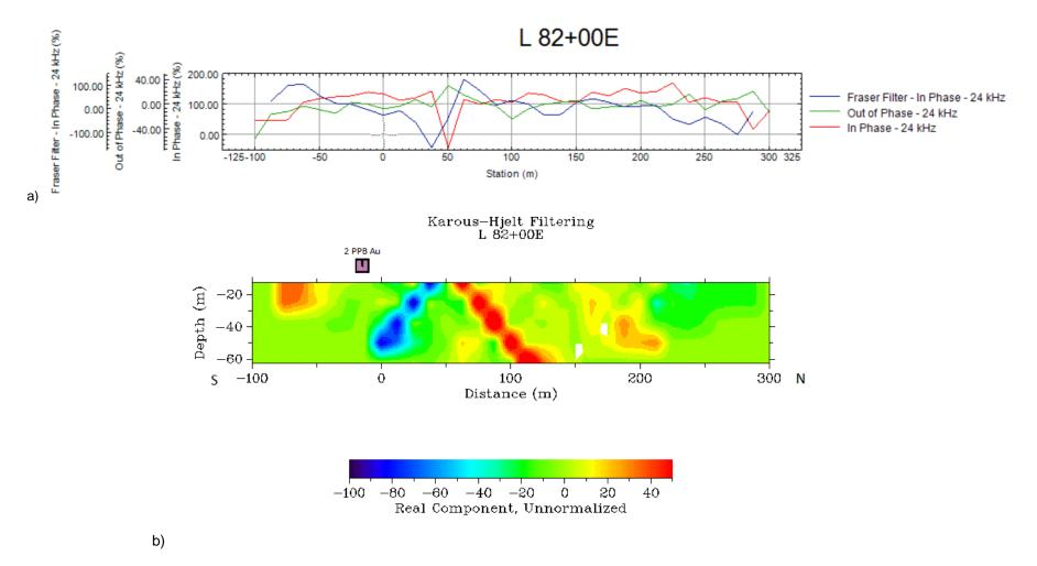
Figure 20. In-Phase, Out-of-Phase and Fraser Filter Profiles (a) Current density Pseudo-distributions obtained with Karous-Hjelt filter (b) – Unnamed Lake – L 82+00E.
