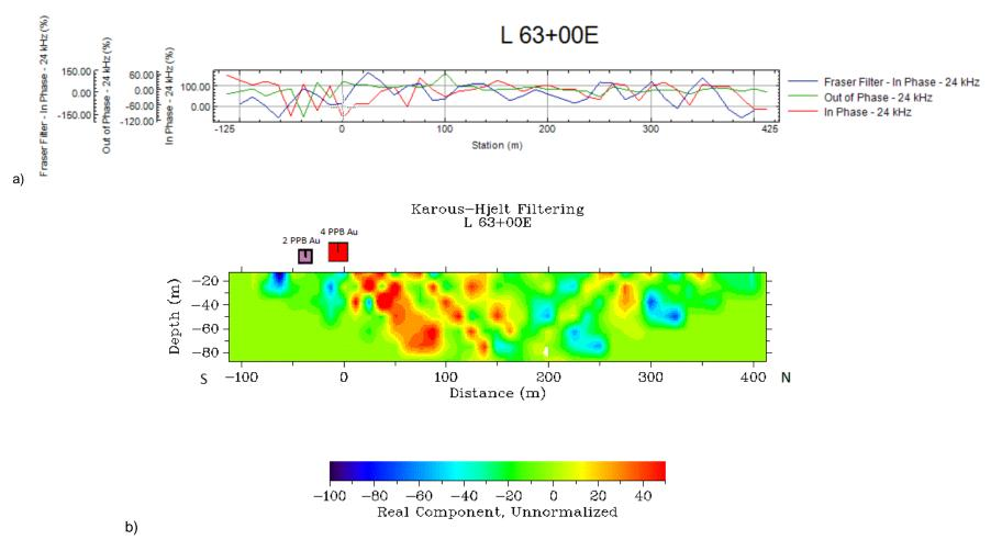
Figure 13. In-Phase, Out-of-Phase and Fraser Filter Profiles (a) Current density Pseudo-distributions obtained with Karous-Hjelt filter (b) – LinJog Lake – L 63+00E.
