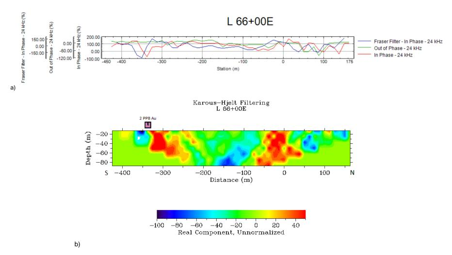
Figure 15. In-Phase, Out-of-Phase and Fraser Filter Profiles (a) Current density Pseudo-distributions obtained with Karous-Hjelt filter (b) – LinJog Lake – L 66+00E.
